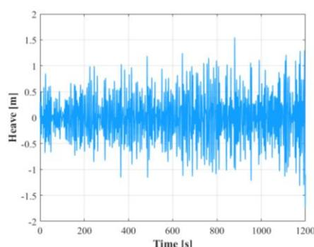
Figure 2. Heave measurements at heading angle of  $180^\circ$
