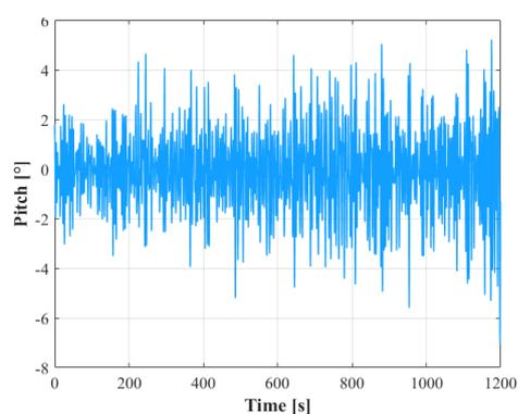
Figure 3. Pitch measurements at heading angle of  $180^\circ$
